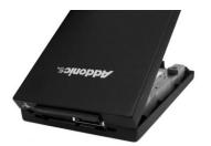
**Step 7** Lower the front of the top cover and making sure the two covers lined up properly. Tighten the small retaining screw on the front of the bottom cover to close the enclosure.
